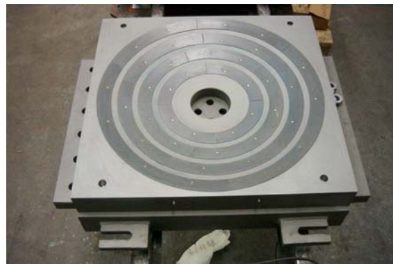
Fig. 2: Bearing bottom or middle section resp. where the spherical part is fixed onto. The concave surface is fitted with a special sliding partner sliding against the chromium plated surface of the spherical part.
