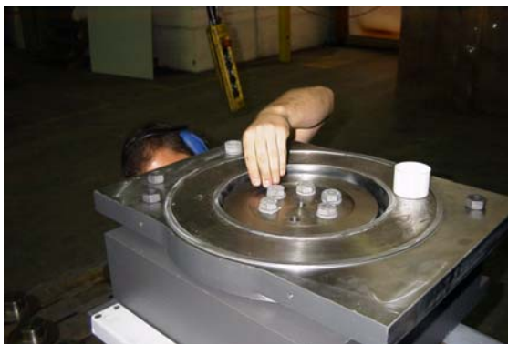
Fig. 3: The spherical part is set onto the bearing bottom or middle section resp. and fixed by the rotation up-lift device set through the hole of the spherical part.
