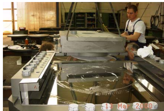
Fig. 4: The package spherical part + bearing bottom or middle section resp. is pushed up-side-down (better assembly!) into the external claws fixed to the top sliding plate also lying up-side-down.
